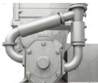
SuperPump SP 290 showing double pump discharge.
